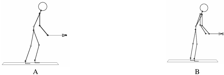
FIGURA 6: Postura assumida durante a alimentação na seccionadora (A) e serra circular (B). FIGURE 6: Adopted posture during feeding in the cutter (A) and circular saw (B).
